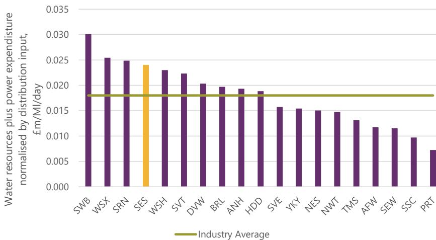
Figure 3.2: Power Expenditure per DI in WRP, Average between 2011/12 – 2022/23
